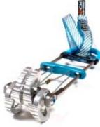
Rock Empire Robot #3 Email to a friend Four cam unit rated to 15kN. Fits cracks 35 to 53 mm (1.38 - 2.08 in.) wide. Weighs 145g.
